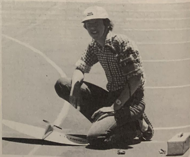
Ron Lumsden prior to the Nats FAI Team Race final. All finalists used Nelson engines, pressure refuelling via multi function valve and either half moon or Russian platform wings. Wilson photo.
