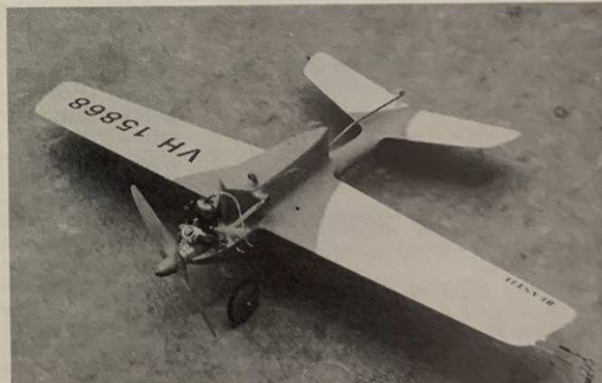
Joe Snaith's 1st place Mouse Racer showing hot finger contacts and overflow prime. Total weight - 7.5 oz.; wing area - 45 sq. in.; tail area 14 sq. in.; Cox TD 049; tank capacity - 23 cc; prop - 5x4 own design glass-epoxy. Other wins include 1980 and 1981 NSW State Champs. Snaith photo.
